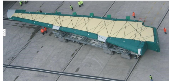
GOETTING equipped wire guided specialty vehicle transporting airplane wing at Airbus Industries
