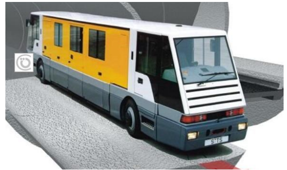
GOETTING equipped wire guided service and emergency evacuation vehicles operating with passengers at the Channel tunnel connecting England with France. Top speed 55 mph, tunnel length 31.4 miles.
