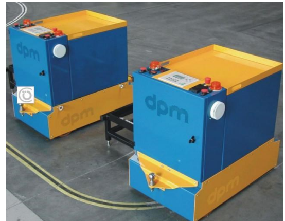
Optical guided AGV by DPM Daum Partner Maschinenbau, Aichstetten Germany
