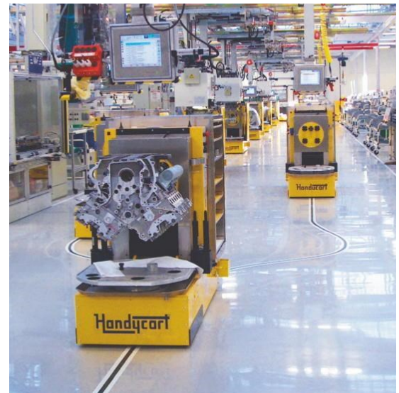
Optical guided AGV by DPM Daum Partner Maschinenbau, Aichstetten Germany
