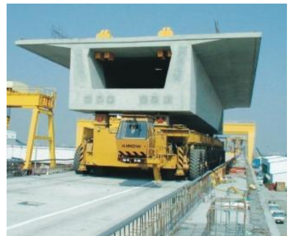
Optical Guided Kirow Multi Mover bridge transporter for elevated highway by Kirow, Germany
